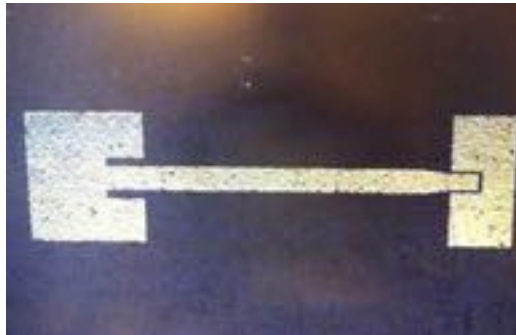
Dummy circuit & LNA on Kapton
