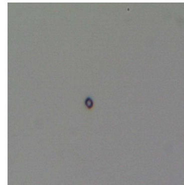
1 \mu\text{m} sized hole in resist!
